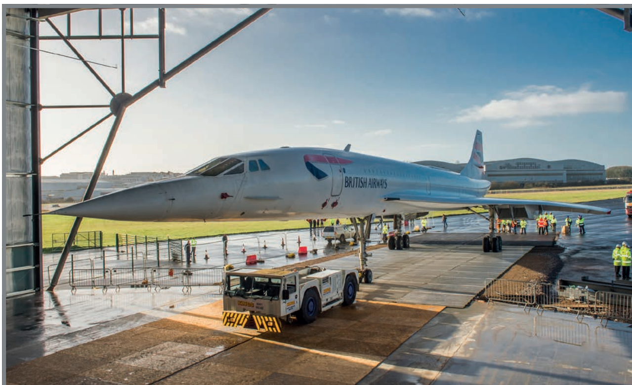
Concorde 'Alpha Foxtrot' being moved into a specially built hangar, at Aerospace Bristol. The hangar was constructed with a movable end wall in order to allow this large aircraft to be placed inside.
