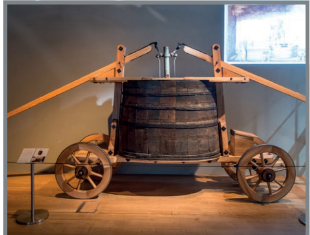
Authenticity: This reconstruction of a 17 Century Fire Engine, contains a historic central barrel and iron pumping mechanism. Based on an early photograph and an original drawing, the Museum of London was able to rebuild the engine to show how it looked and how efficiently it worked.
