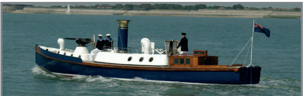
Steam Pinnace 199 was built in 1911 and it is believed to be the last remaining operational naval picket boat. The Pinnace is part of the collection of the National Museum of Royal Navy. Between 2012-2015 and over 13,000 hours of work, volunteers completed a major refurbishment of the hull, replacing cracked beams and rotten timbers including a section of the keel, the hog and part of the stern. The boiler was re-tubed with all valves overhauled and all auxiliary machinery inspected and repaired. After completion in 2015, the project won the Icon Conservation Award for Volunteering in the Conservation of an Industrial Heritage Artefact, awarded by The Institution of Mechanical Engineers.
