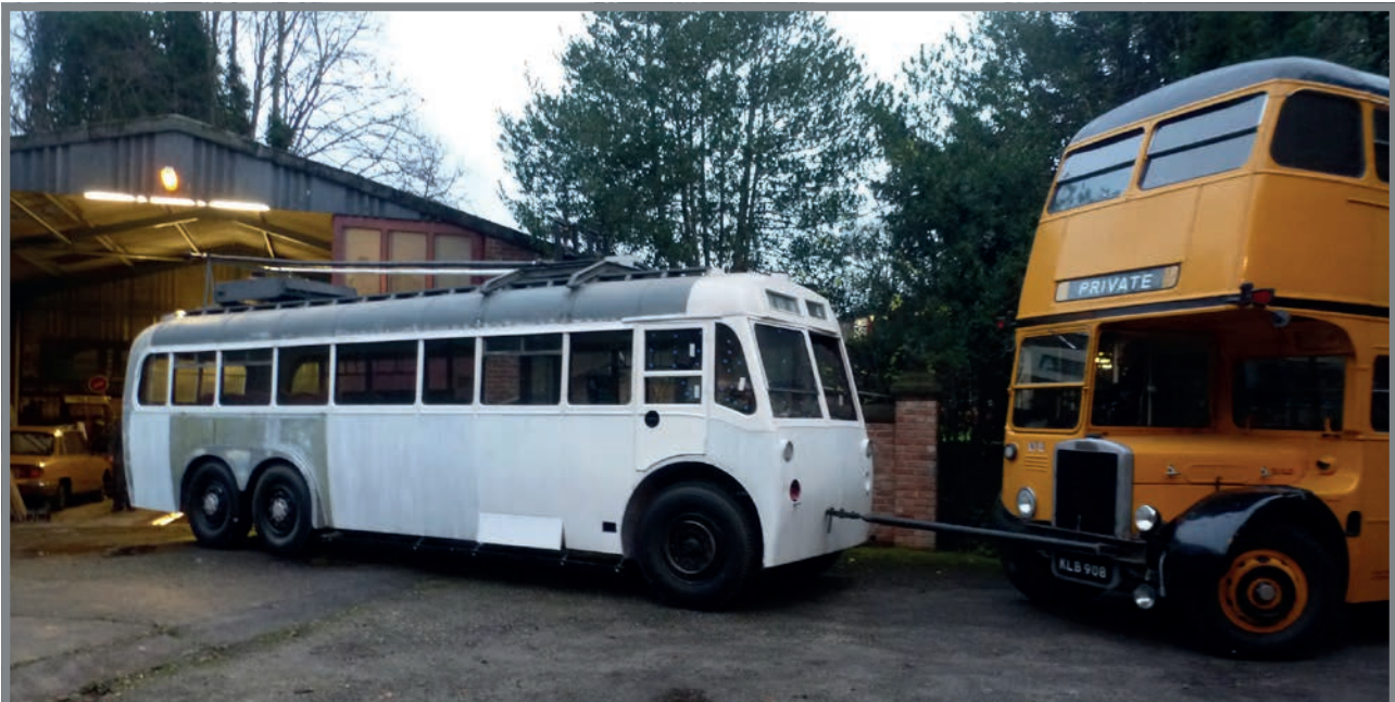
A 1942 Sunbeam Trolleybus, with its exterior panelling restored and primed, awaiting repainting.
