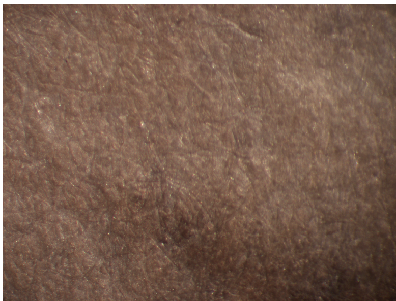
Figure 15 Paper fibers visible under the albumen layer of a photograph examined using a high-power loupe or microscope (80× magnification).
