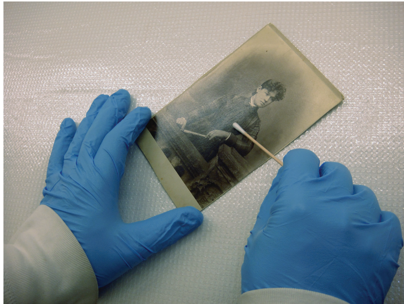
Figure 34 Dry swabbing of the surface of a photograph to determine the presence of albumen using ELISA.
