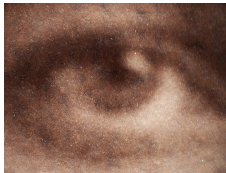
Figure 14c Micrograph showing an absence of microcracks, as is typical of burnished albumen prints in fig. 13 recorded at 40× magnification.
